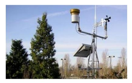
Get accurate, up to-the-minute weather and climate information from the five Lake Oswego weather stations. Currently all stations record and display temperature, rainfall, wind speed and direction, relative humidity, dew point, soil moisture content, soil temperature and evapotranspiration (ETo).
