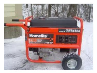
Portable generators are useful during power outages. However, many homeowners are unaware that the improper use of portable generators can be risky. The most common dangers associated with portable generators are carbon monoxide (CO) poisoning, electrical shock or electrocution, and fire hazards.
