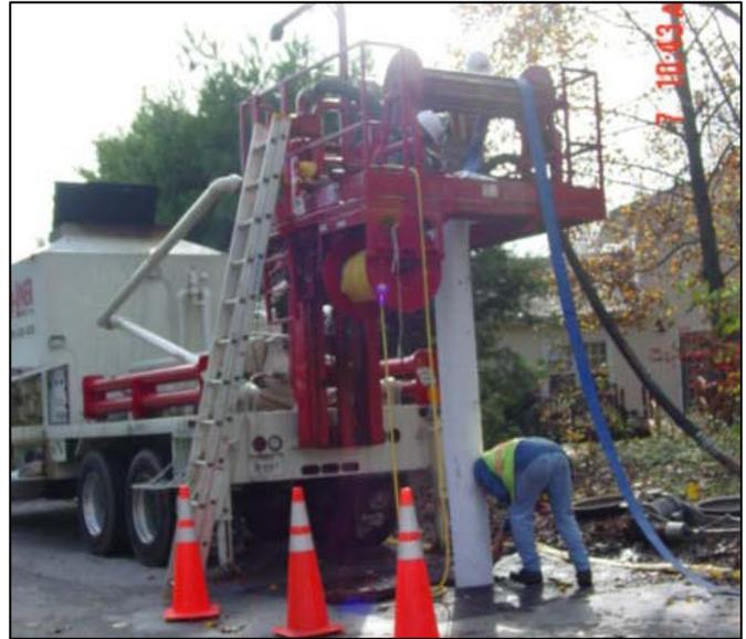
*Truck mounted boiler for installing CIPP*
