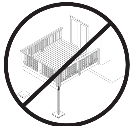
Fig. 11: No attachment to house overhang
